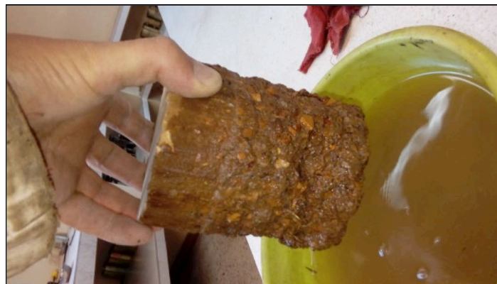
Figure 6. Water stability test after 30 minutes. Source: provided by the authors
