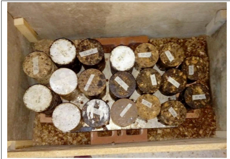
Figure 12. Chamber for curing specimens. Source: provided by the authors
