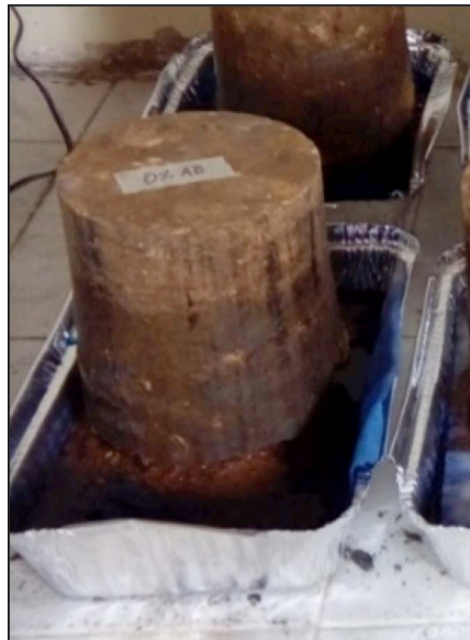
Figure 5. Briquettes after the capillary absorption test. Source: provided by the authors
