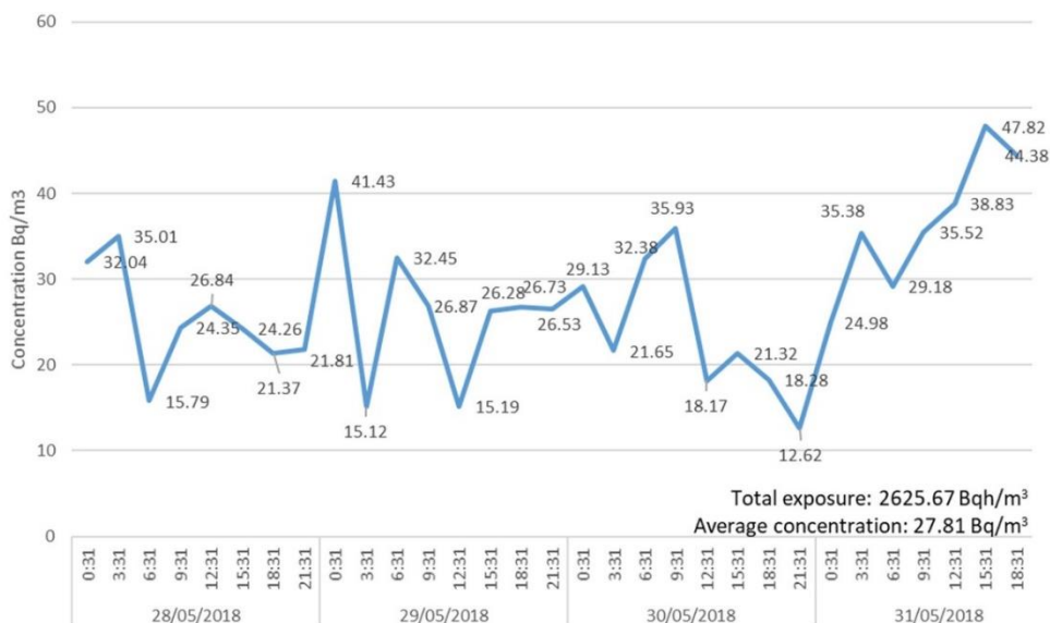
Figure 9. Data obtained in the living room on the ground floor with ventilation.
