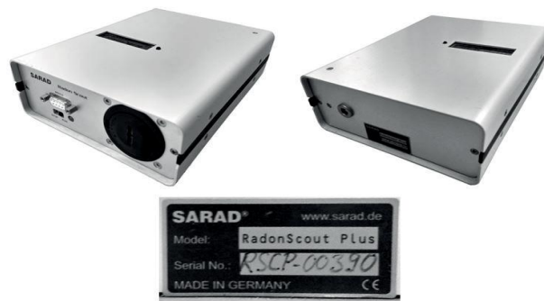
Figure 4. Instrument used to collect Radon data.
