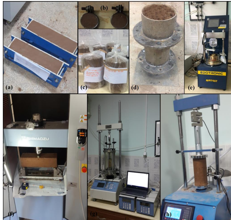
Figure 4. Sample preparation and experiments; (a, b, c) prepared samples, (d) segregation test, (e) consolidation test, (f) three-point flexural test, (g) triaxial test, (h) unconfined compression test.
