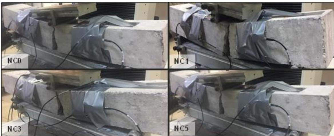
Figure 4. Failure of the test specimens after center-point-bending test.
