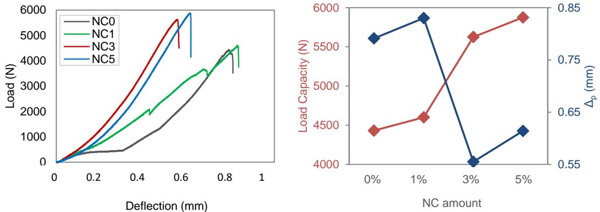
Figure 3. a) Load vs. deflection curves, and b) load vs. deflection relations at ultimate load levels.
