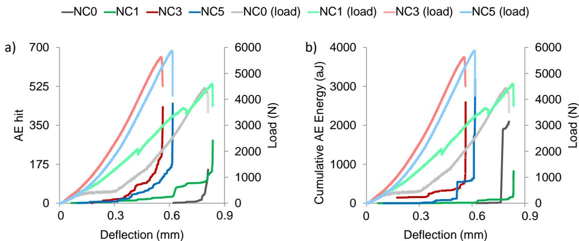
**Figure 5.** a) AE hits, b) cumulative AE energies.
