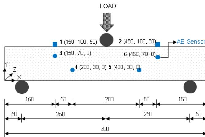
**Figure 2.** Center-point-bending test configuration and AE sensors (mm).
