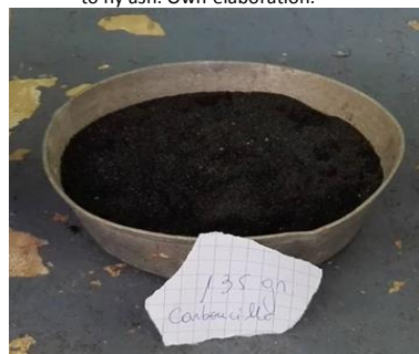
Figure 1. Unburned carbon extracted and dried after the wash treatment to fly ash. Own-elaboration.
