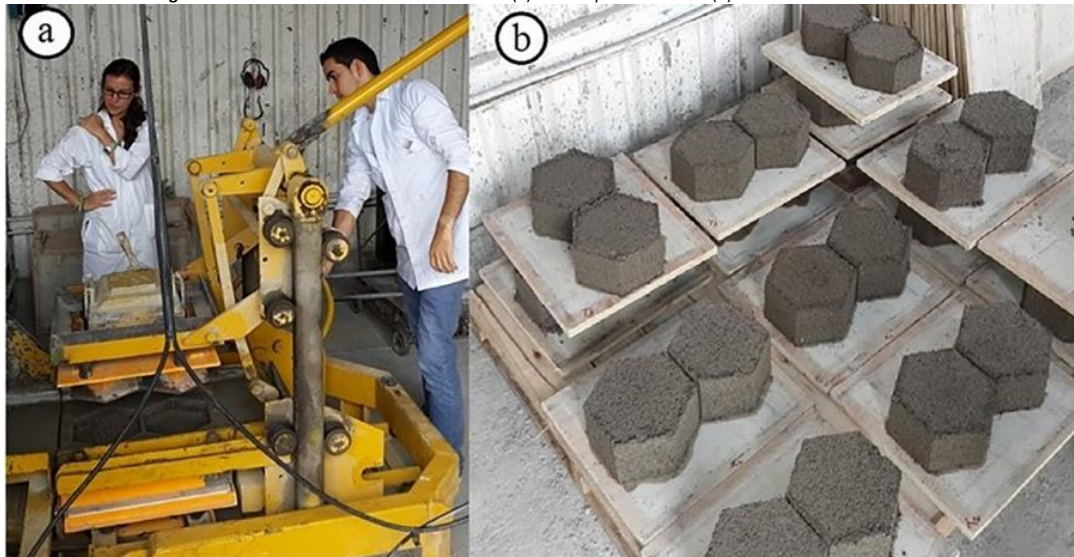
Figure 1. Machine used to manufacture blocks (a) and shape of the block (b). Source: Self-Elaboration.
