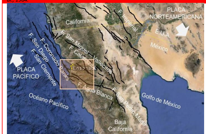
Figure 2. Seismotectonic framework; major systems associated with the interaction of the Pacific and North American plates faults. Modified from Kahle et al., 1984.
