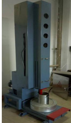
Figure 4. The numerical control multi-functional compaction test apparatus. (Self-Elaboration).
